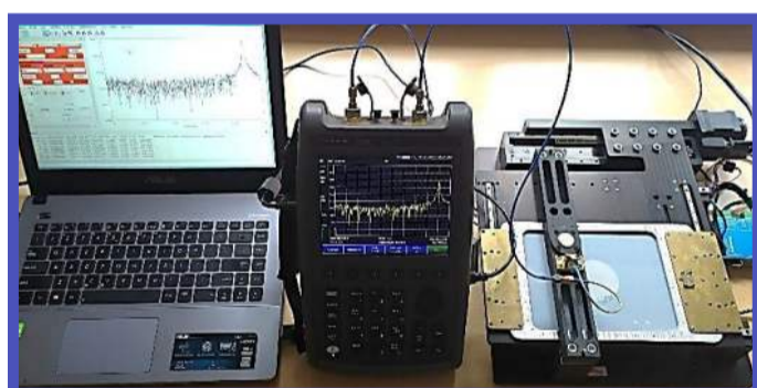
A photo of the imaging system built of the 2D SPDR scanner
